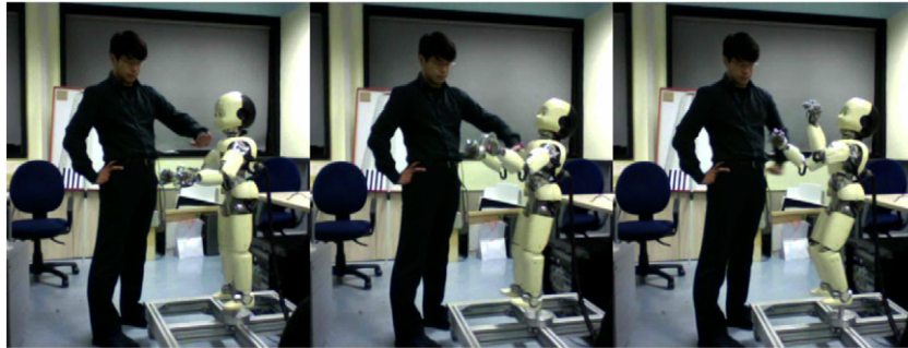
Fig. 16. Learning phase of the upper arm collision with experimenter (A). Only the front reaction of the right arm was stopped by the tonic reflex.
