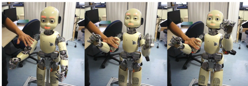
Fig. 14. Collision detection and the tonic reflex elicitation.
